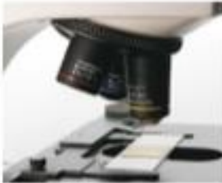
Figure 6: Some microscopes have a slide holder rather than clips. This grips the sides of a slide and allows fine movement of the slide on the stage.
